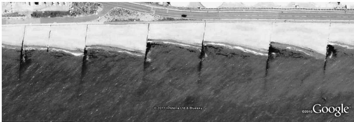
Figure 1: A plan view of a typical timber groyne field showing a saw-tooth beach plan shape
