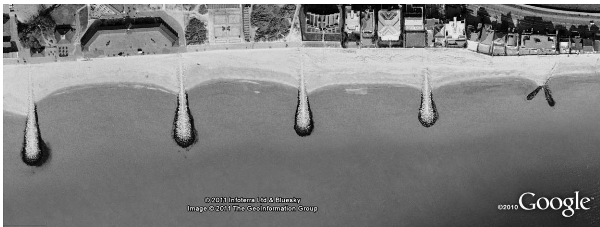
Figure 2: A plan view of a typical rock groyne field showing a curved beach plan shape
